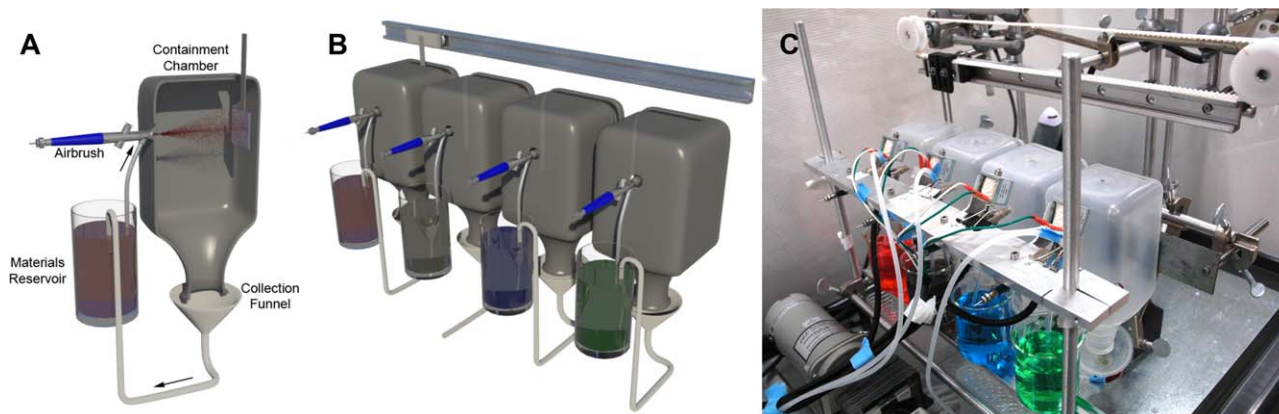
Figure 1. Representative designs of the spray LbL setup with the modifications employed in this study. The cross-sectional view of one of the containment chambers (A) shows that for deposition, the solution is aerosolized onto a substrate and then collected for its return to the materials reservoir via peristaltic pump. In multilayer assembly, the substrate is positioned and coated in a pre-programmed sequence among four solution-specific chambers (B). The actual setup is capable of fitting on the standard laboratory bench (C). [Color figure can be viewed in the online issue, which is available at wileyonlinelibrary.com .]
